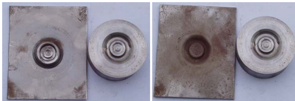
Fig. 10 Results of forming of a 2.5-mm thick ductile steel sample against a medium die M2. Die side ( left ), and impact side ( right ) views
