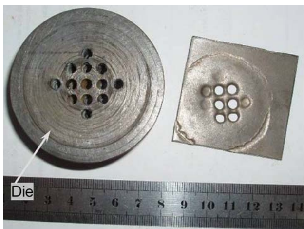
Fig. 7 Formation of the multiple openings by a single impact of a round jet. Steel sheet thickness is 2.5 mm and the opening diameter is 4 mm. Notice that the liquid penetration into the workpiece can be controlled by the impact condition
