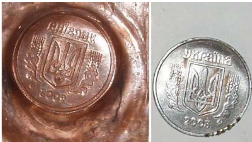
Fig. 18 General view of a coin stamped on copper and original coin used as a die. Notice reproduction of fine details of the coin on the sample surface
