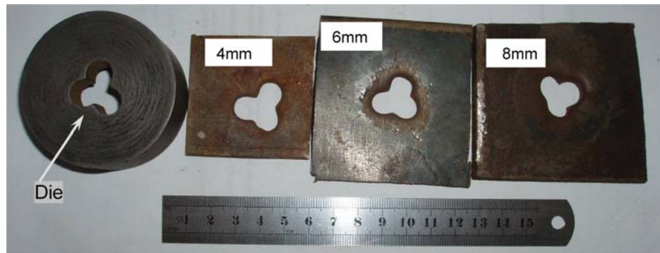
Fig. 5 Formation of shaped openings using a round jet. Notice that the workpiece thickness does not affect the accuracy of the piercing
